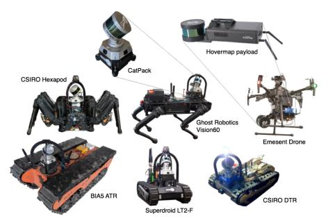
**Figure 1.** Team CSIRO Data61 deployed a set of heterogeneous ground and air robots, with homogeneous sensing payloads. *Top Row*: CatPack and Hovermap modular sensing payloads, both using a rotating lidar system for the UGVs and UAVs. *Middle Row*: CSIRO Hexapod, Ghost Robotics Vision60 quadruped, and an Emesent UAV with the Hovermap payload. *Bottom Row*: BIA5 All Terrain Robot (ATR), SuperDroid LT2-F, and CSIRO Dynamic Tracked Robot (DTR).
