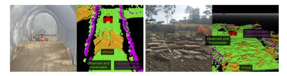
**Figure 13.** Examples of 2.5D cost maps generated for a bump in a tunnel on the left and a slope unevenly embedded with stone steps on the right. Green cells have been directly observed and are possibly traversable, pink cells have been directly observed and are definitely not traversable, and orange cells have not been observed but are best case height estimates called virtual surfaces.
