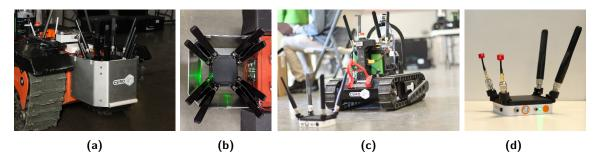
**Figure 9.** Drop nodes from the Urban Circuit: Rajant ES-1s were modified to contain a battery and hold the antenna upright. (a) and (b) show a five node dropper "stack" attached to the back of the ATR. (c) shows a single node deployed from a SuperDroid robot. (d) shows a single Rajant node.
