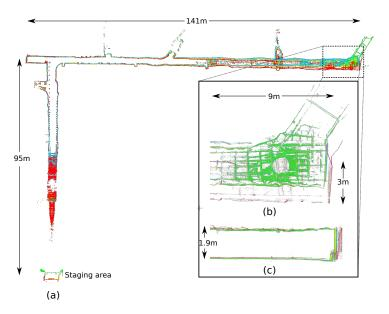
**Figure 22.** The point cloud map from a single UGV for the Safety Research Mine course with a total transit of approximately 215 m overlaid with the SLAM solutions and reference map. Approximate cross-section measurements are supplied for reference. Red, odometry; blue, Atlas (real time); yellow, global (offline); green, reference point cloud provided by DARPA. (a) Top orthographic projection showing the entire map. (b) Top orthographic projection showing the end of the map.
