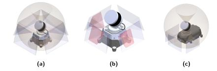
**Figure 2.** The CatPack showing FOV of the lidar and RGB cameras for the newer configuration utilized in Tunnel, Urban, and Cave events in (a), with the thermal camera FOV shown in red in (b) and the older configuration utilized in STIX with narrow FOV RGB cameras in (c).
