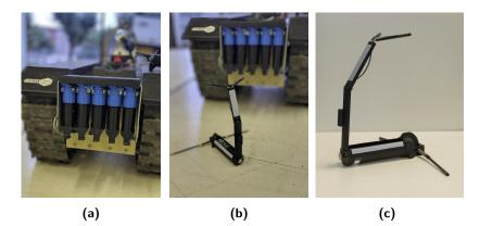
**Figure 8.** Ubiquiti drop nodes, as they were carried in the node dropper at the back of the ATR (a), a self-erected node after being dropped (b), and another view of the deployed drop node that consists of the Ubiquiti radio, a LiPo battery, a servo motor, and the circuitry to perform delayed self-righting and erecting the antenna after being dropped (c).
