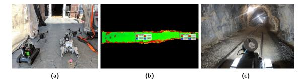
**Figure 20.** Robot team utilized at STIX at starting gate (a), consisting of two Emesent Hovermap UAVs, a SuperDroid LT2-F and a Ghost Robotics Vision60 quadruped prototype (v3.2) automated with modular CatPacks. The Miami Tunnel at STIX constricted to under 2 m width within 30 m of the entrance (b), preventing further exploration with the UAV system. The rails in the Miami Tunnel caused the SuperDroid LT2-F platform to get stuck after traversing 120 m due to its low ground clearance (c).
