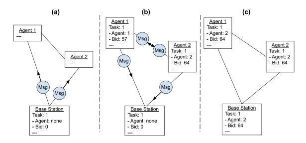
**Figure 17.** Simple consensus example. (a) Operator station sends a drop-node task. (b) Each agent bids and broadcasts its bid across the network. (c) Agents and base station form consensus on who will execute task.
