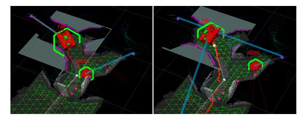
**Figure 18.** *Left:* Two agents distribute tasks to investigate separate areas between themselves. The light-blue lines represent the "task path," the path the agent expects to take as it completes its bundle of tasks. *Right:* One agent is tasked to return home; the other agent immediately picks up the released task to execute itself.
