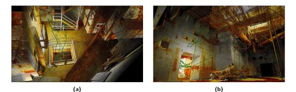
**Figure 25.** Post-processed, intensity-colored point cloud generated from UAV in mission descending through shaft in the beta course, with trajectory overlaid. (a) Upper level where mission commenced, and (b) lower level with trajectory descending through shaft and entering adjacent rooms.
