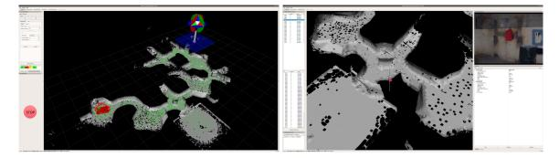
**Figure 19.** *Left:* Command panel of operator GUI with example of operator command input in the form of task prioritization region in blue. *Right:* Object panel of operator GUI with a detection selection from detection list, visualized as a location on the map and the detection image for operator verification and potential report submission.
