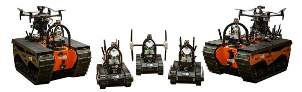
**Figure 23.** The Urban Circuit robot fleet consisted of two BIA5 ATRs each carrying an Emesent Hovermap UAV, and three Superdoid LT2-F platforms.
