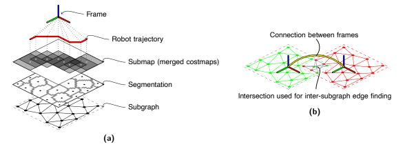
**Figure 16.** Topometric map generation involves (a) derivation of subgraphs from the superpixel segmentation of submaps associated with each root frame, and (b) finding traversable edges between vertices of different subgraphs by inspecting the intersection of submaps from connected frames.
