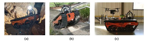
**Figure 6.** BIA5 ATRs (a) traversing challenging terrain during the Cave event, (b) traversing stairs, and (c) carrying UAV deployment platform and communication node dropper utilized at the Urban Circuit event.
