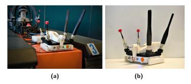
Figure 10. Node droppers from the cave circuit, with (a) showing the new dropper attached to the ATR.
