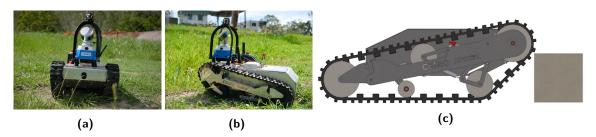
**Figure 7.** CSIRO Dynamic Tracked Robot (DTR) shown in (a) and (b) was designed to overcome stairwells and high steps without the use of a flippers. A CAD drawing of the DTR is shown next to a 180 mm step as reference in (c).
