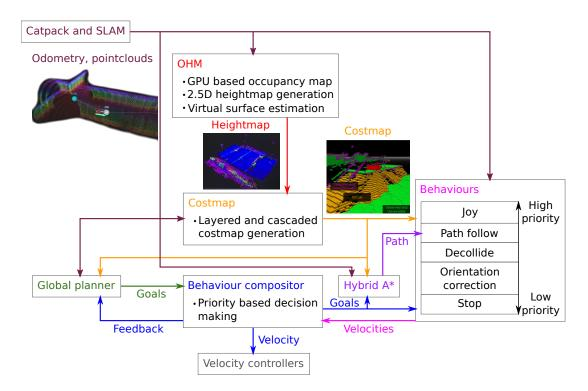
Figure 12. UGV local navigation components and shared information.
