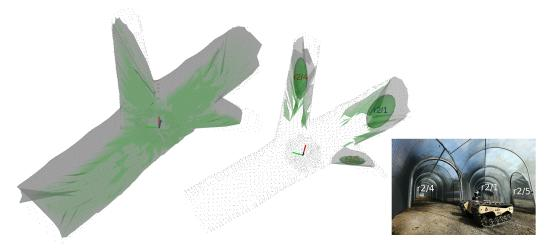
**Figure 11.** Example of frontier processing in CSIRO test tunnel. Left: Watertight mesh of visible space from observer location. Middle: Frontiers identified from agent position, having entered from left. Right: Corresponding image with frontiers labeled.
