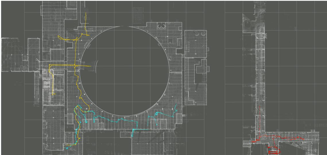
**Figure 18.** Ground truth map of the Alpha course in Urban circuit with upper (left) and lower (right) floors. Robot positions overlaid in colors each representing a different robot during a run 4. 10-m grid.
