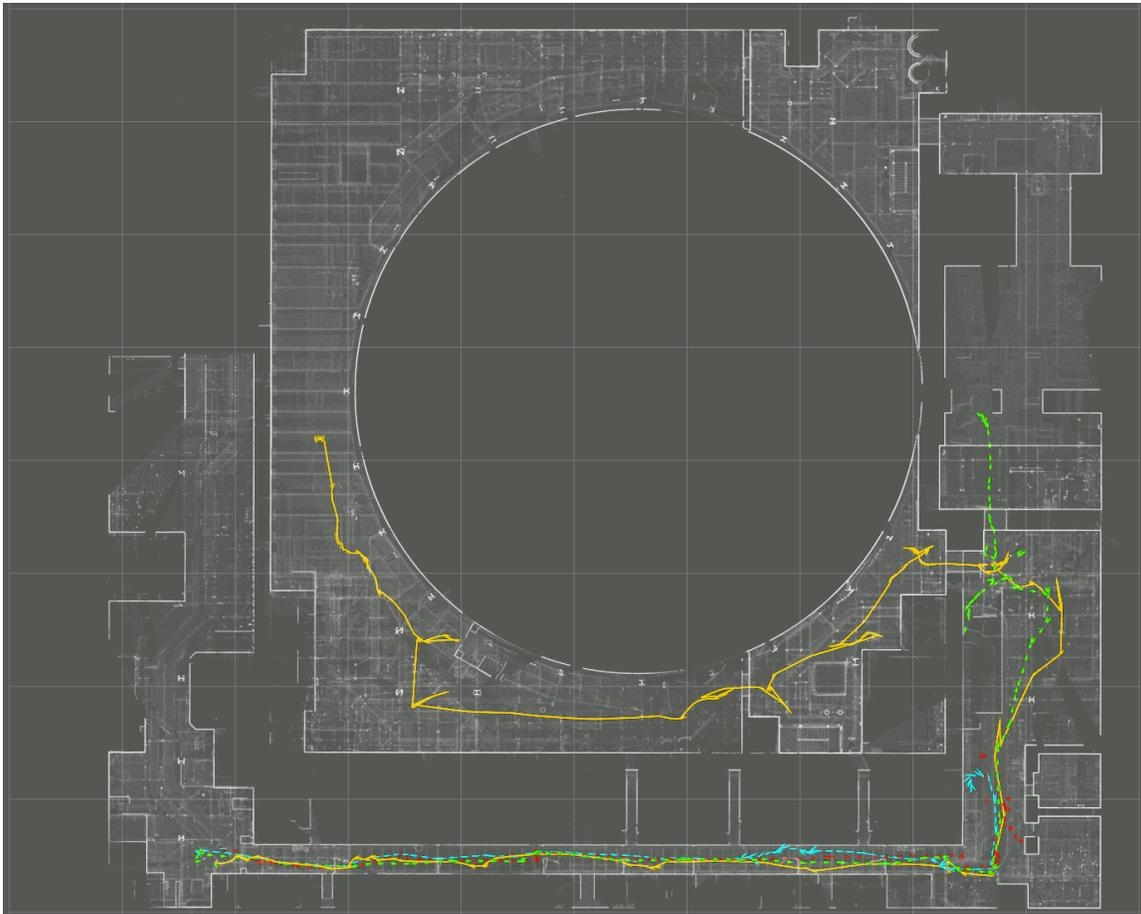
**Figure 17.** Ground truth map of the Beta course in the Urban circuit. Only the top floor since our team was unable to explore any other level. Robot positions overlaid in colors each representing a different robot during a run 3. 10-m grid.
