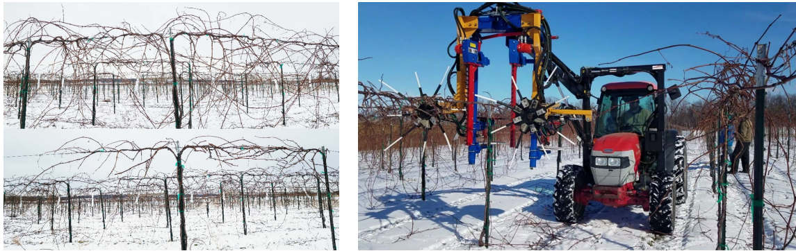
Figure 1. Dormant Concord grapevines before and after mechanical prepruning (left top and bottom) with an OXBO V-Mech sprawl prepruner (right).
